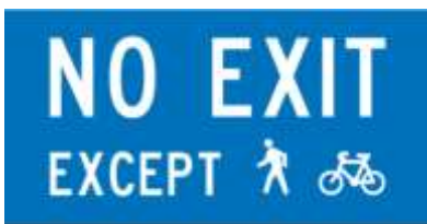
Figure 54: AJ11A (TCD Rule) 'No exit except pedestrians and cyclists' sign
