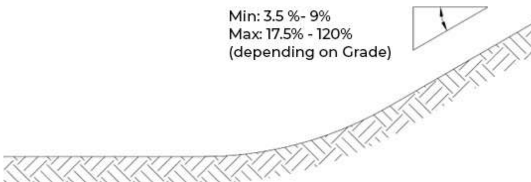
Figure 12: Cross-section for super-elevated (or bermed) turns
