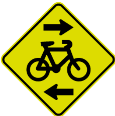
Figure 64: W16-7.1 (TCD Rule) 'Cycle path – crossing' permanent warning sign for motorists
